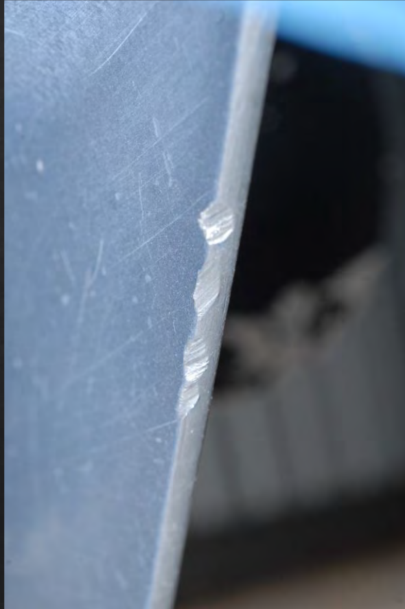
Damage to shaft
